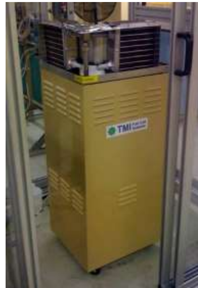
1 kilowatt SOFC genset operating at Lockheed Martin, running on DoD standard JP-8 fuel
